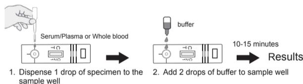
Read the instruction first prior to testing. Bring the pouched test to room temperature prior to testing. Do not open the pouch until ready to begin testing.
